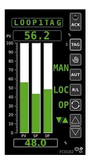
The *Panelicity*® displays feature intuitive icons for navigating menus compared to traditional 3x6 controllers. Typical setup parameters such as I/O types, ranges, and PID parameters are logically organized with no need to learn special software. Up to 5 alarms and 5 digital outputs can be defined for each control loop. Control templates have a data entry table to document your settings for back-up. Security access authority is provided to eliminate unauthorized field changes.
