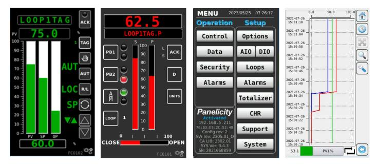
The **Panelicity**<sup>®</sup> displays feature intuitive icons for navigating menus compared to traditional 3x6 controllers. Typical setup parameters such as I/O types, ranges, and PID parameters are logically organized with no need to learn special software. Control templates have a data entry table to document your settings for back-up. Security access authority is provided to eliminate unauthorized field changes.
