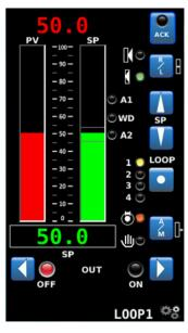
The *Panelicity*® displays feature intuitive icons for navigating menus compared to traditional 3x6 controllers. Typical setup parameters such as I/O types, ranges, and PID parameters are logically organized with no need to learn special software. Control templates have a data entry table to document your settings for back-up. Security access authority is provided to eliminate unauthorized field changes.
